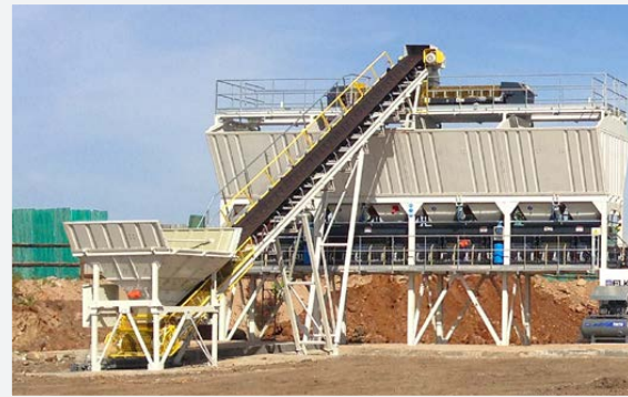
Shuttle Type Automated Aggregate Feeding System
