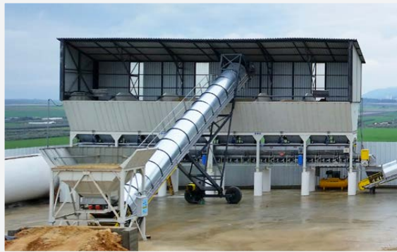
Radial Type Automated Aggregate Feeding System
