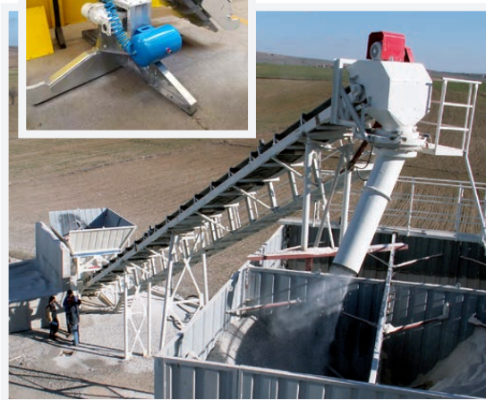
Bottom drive new distribution system with pneumatically activated flap
